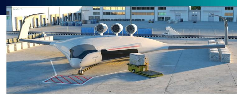
Natilus is currently developing three products, all with carbon-fiber composite airframes. The first is a 19,000-pound aircraft with a 90-foot wingspan, slated to begin production late in 2021. The second is a 60-ton aircraft, similar in size to a Boeing 767, targeted for domestic service in the U.S. but also capable of serving Europe and Asia. The flagship product is a 700-ton competitor to the Boeing 777 with 10 percent larger wingspan, capable of trans-Pacific flight.
