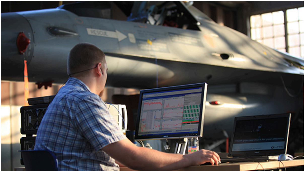
Ground vibration testing: modal test on the full aircraft structure as part of the certification process.
