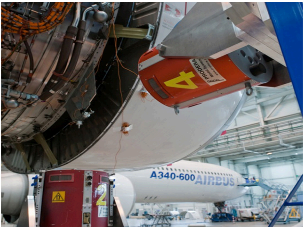
Lateral and vertical exciters placed on the aircraft engine during the certification of the A340-600 (images courtesy of Airbus, Onera and DLR).
